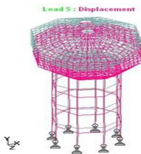
Fig.6: Tank with Its Full Capacity by Considering Only Hydrostatic Forces.
