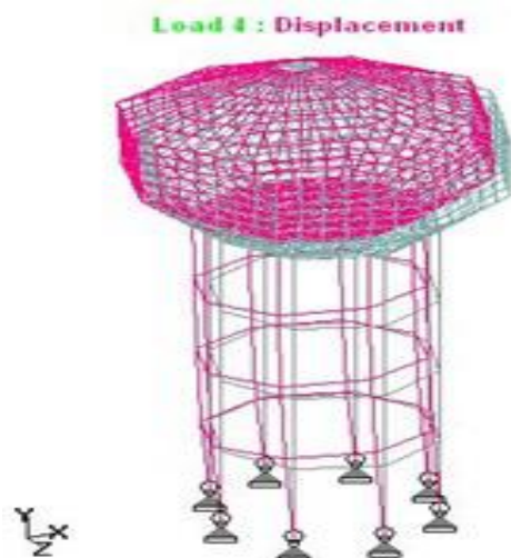
Fig.7: Tank with Its Full Capacity Considering Hydrostatic Forces Along with Sloshing Forces in the Tank
